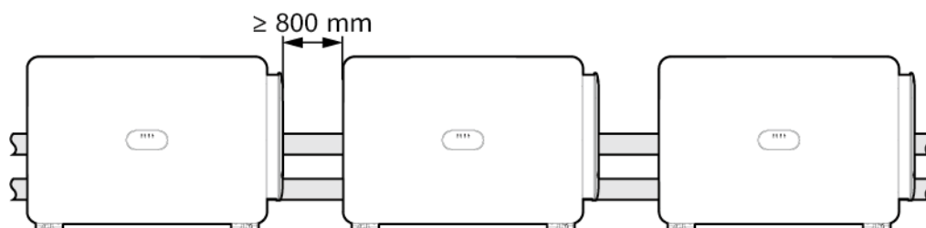
Figure 4-5 Horizontal installation mode (recommended)
