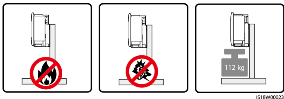
Figure 4-2 Mounting structure requirements
