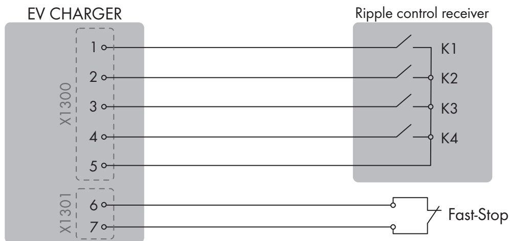
Figure 15: Connection of a Ripple Control Receiver
